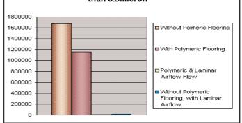
Figure 1. Airborne particle (<0.5 microns) counts recorded under different test conditions (see text)
