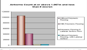
**Figure 2.** Airborne particle (<5 microns) counts recorded under different test conditions.
